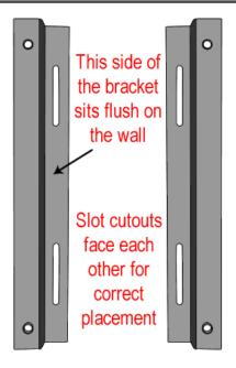
Place a bracket with the slotted side flush on the wall and the slots facing toward the center of the fireplace. Line up the anchors vertically in the slot cutouts. Place an anchor screw through the bracket slot into the anchor and tighten. Do not over tighten as you may strip the wall anchor. Do this for both brackets.
