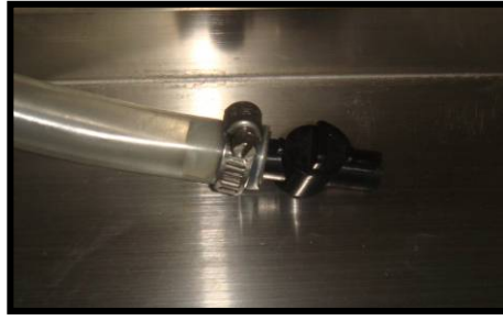
B. Flow Control Valve (Inside Reservoir)
