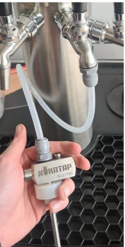
The NukaTap counter pressure bottle filler can also be used to bottle directly from a pressurised FermZilla or keg.
