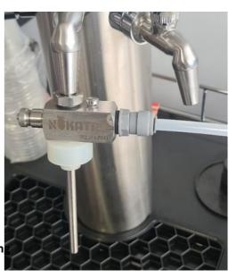
Connecting to a regulator via a quick disconnect and EVABarrier Hosin
