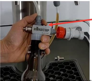
Secure the bottle against the stopper and purge the headspace for a few seconds
