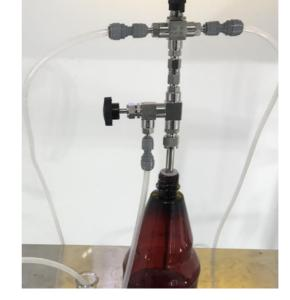
**Step 5.** Start with the handle of the counter pressure bottle filler in the off position (perpendicular to
