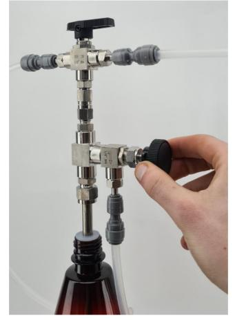
**Step 8.** After the bottle has been purged of any oxygen, close the bleed valve and pressurise the bottle back up to 10psi with CO2.
