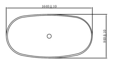
Net Weight: 91 kg Gross Weight: 131 kg Water capacity: 330 L
