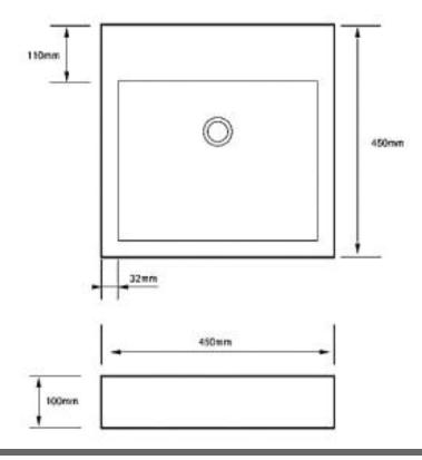
Net Weight: 15kg Gross Weight: 18kg Unit: mm
