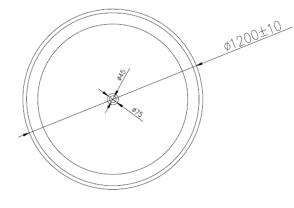
Net Weight: 122kg Gross Weight: 172 kg Water capacity: 528 L Unit: mm (10mm tolerance)
