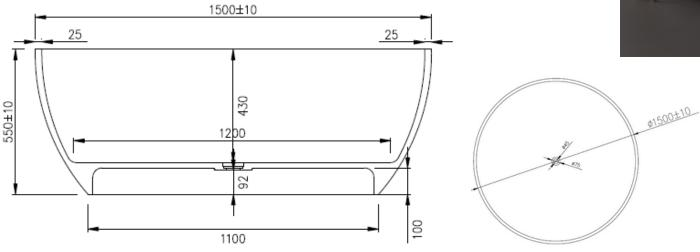
Net Weight: 149kg Gross Weight: 199kg Water capacity: 660L Unit: mm (10mm tolerance)
