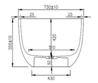
Net Weight: 96kg Gross Weight: 146kg Water capacity: 194L Unit: mm (10mm tolerance)
