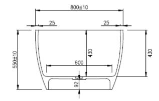
Net Weight: 129kg Gross Weight: 179kg Water capacity: 338L Unit: mm (10mm tolerance)
