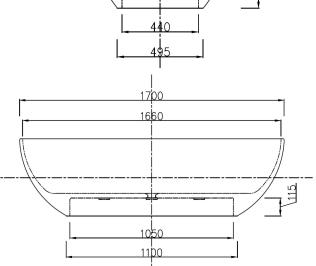
Net Weight: 132 kg Gross Weight: 182kg Water capacity: 300L
