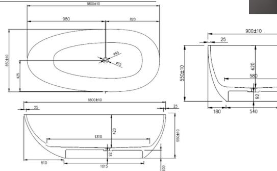
Net Weight: 123 kg Gross Weight: 173kg Water capacity: 328L
