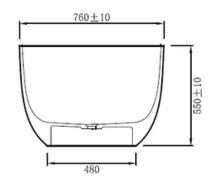
Net Weight: 79 kg Gross Weight: 129 kg Water capacity: 208 L Unit: mm (10mm tolerance)
