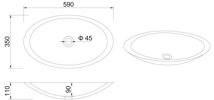
Net weight: 6.5 kg Gross weight: 8.5 kg Unit: mm
