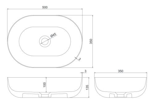
Net weight: 8.3kg Gross weight: 10kg Unit: mm
