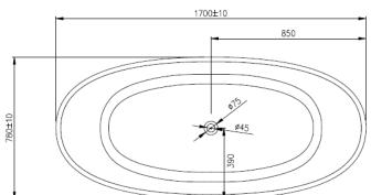
Net Weight: 116 kg Gross Weight: 166 kg Water capacity: 238 L
