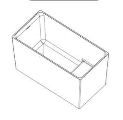
Net Weight: 150kg Gross Weight: 200kg Water Capacity: 320L Unit: mm
