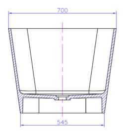
Net Weight: 125kg Gross Weight: 275kg Water Capacity: 250L
