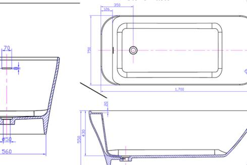
Net Weight: 135kg Gross Weight: 185kg Water Capacity: 272L
