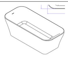
Net Weight: 135kg Gross Weight: 185kg Water Capacity: 275L Unit: mm
