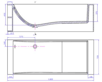
Net Weight: 170kg Gross Weight: 220kg Water Capacity: 280L
