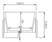
Net Weight: 149kg Gross Weight: 199kg Water capacity: 338L Unit: mm (10mm tolerance)
