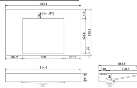
Net Weight: 26kg Gross Weight: 27kg Unit: mm 5-10mm tolerance
