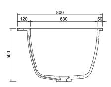
Net weight: 120kg Gross weight: 190kg Water capacity: 280L
