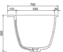
Net weight: 112kg Gross weight: 174kg Water capacity: 220L
