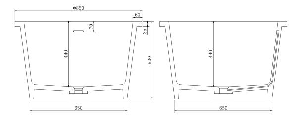
Net weight: 136kg Gross weight: 176kg Water capacity: 90lt Unit: mm
