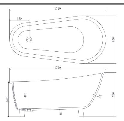
Net weight: 165kg Gross weight: 250kg Water Capacity: 275lt Unit: mm
