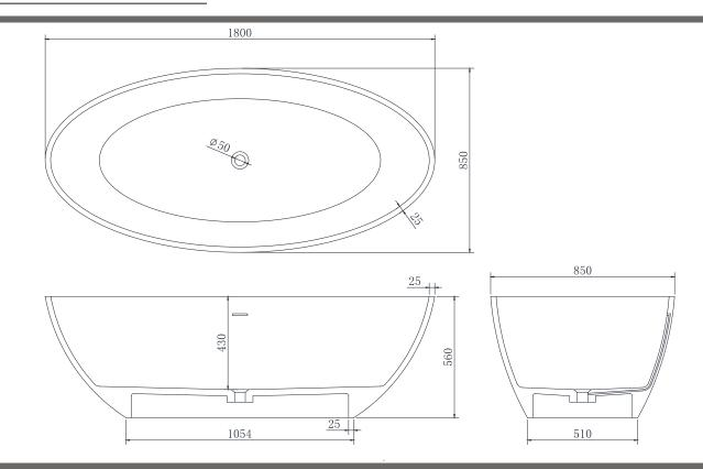
Net weight: 158kg Gross weight: 233kg Water Capacity: 238lt Unit: mm
