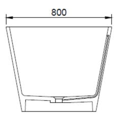
Net Weight: 155kg Gross Weight: 232kg Water capacity: 420L
