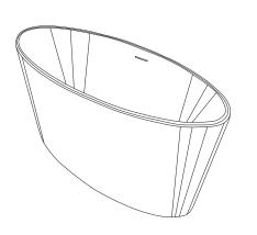
Net weight: 135kg Gross weight: 192kg Water capacity: 200L Unit: mm
