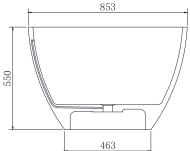
Net weight: 168kg Gross weight: 238kg Water Capacity: 255lt
