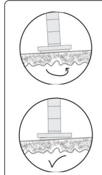
**A**—For sloping floors rotate Stump Base to level Monkee Tree
