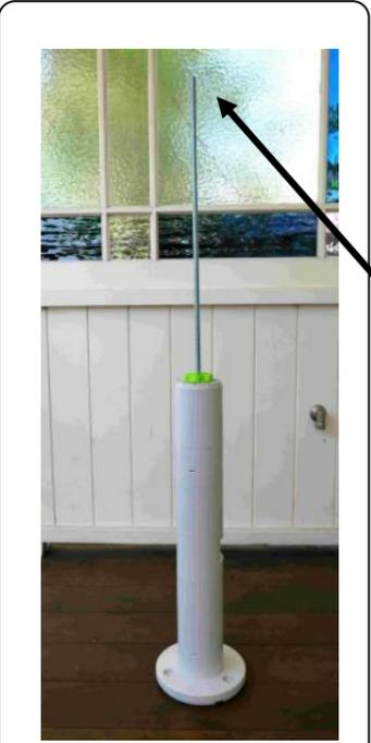
**C**- Add next rod ensuring slot is at top. Use coin or wall brackets & slot to tighten rod.
