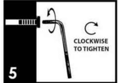
Finally, make sure all parts are properly aligned then use the included **tools** to completely tighten the screws. Your furniture is now ready for use.
