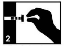
Position each part correctly and insert all screws into their respective holes. Then, **hand-tighten** only until 70% tight. Complete tightening with the tools will come at a later step.
