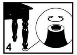
Some furniture come with optional height adjustment knobs underneath each leg. Turn this knob counterclockwise to raise the leg level or dockwise to lower the leg level.
