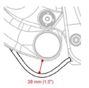
If there is too much slack push the cable up into the downtube gently, do not push the cable into the rear triangle as it will cause the cable to rub against your spokes. If there is not enough slack gently pull the cable out of the downtube to 38mm (1.5"). After adjusting your cables be sure to check the cable clearance between your brake cable and wheel.
