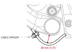
If there is to much slack push the cable up into the downtube gently, do not push the cable into the rear triangle as it will cause the cable to rub against your spokes. If there is not enough slack gently pull the cable out of the downtube to 38mm (1.5"). After adjusting your cables be sure to check the cable clearance between your brake cable and wheel.
