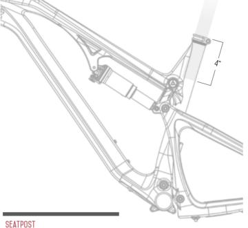
MAKE SURE TO INSERT SEAT POST AT LEAST 4" INTO THE MAIN FRAME. ANYTHING LESS THAN THIS AMOUNT COULD CAUSE DAMAGE TO THE FRAME OR EVEN FAILURE.
