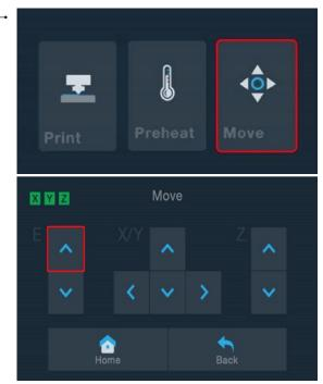
14. If the Main Menu is displayed, touch the **Move**button to enter the Move Menu. If already on the Move Menu, touch the button (enclosed in red in the image below) to start feeding filament into the extruder. Continue touching the button until several centimeters of filament have been extruded.
