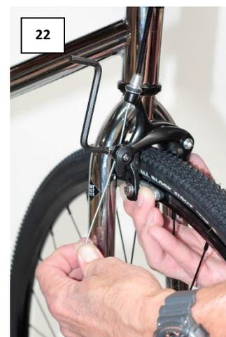
Be sure that the brake arms are evenly spaced from the wheel and there is some clearance between the brake pads and the rim surface. If the arms are not evenly spaced from the wheel, you can balance the spacing by gripping the brake assembly and rotating until it is centered with the wheel
