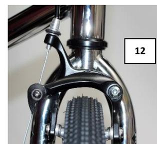
5 - Close the lever the rest of the way until it is pointing towards the back of the bike. There should be considerable resistance from the lever when closing it all the way (**Figure 11**). If there is too much or too little resistance, adjust by loosening or tightening the adjusting nut until the desired resistance is reached.
