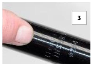
**WARNING!** *Using the bike with the minimum insertion line on the lower portion of the seat post showing above the frame could result in a failure of the seat post and/or the frame causing a loss of control with potential injury to rider.* Such failures are not covered by warranty as it is improper use of the product. (**Figure 3**)
