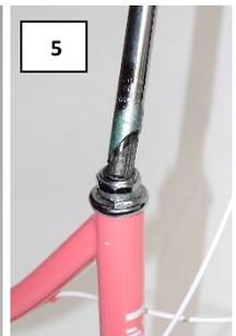
4. Adjust the height of the stem to your desired level and tighten the stem bolt using a 6mm wrench. You can make final adjustments to the height of the stem after the bike is assembled. NOTE: *Be sure that the minimum insertion mark on the shaft of the stem is inside the frame, it must not be visible outside of the frame.* (**Figure 6**)
