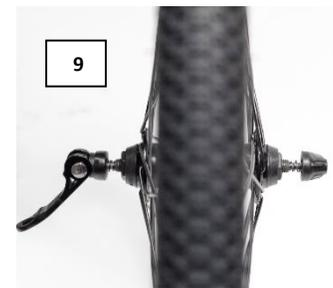
4 - Test for proper adjustment by closing the Quick Release lever. When properly adjusted, the lever should begin to clamp the fork at approximately the half way point of lever travel (**Figure 10**). If the lever clamps the fork drop out before or after the halfway point of the lever travel, adjust by loosening or tightening the adjusting nut until the desired adjustment is reached.
