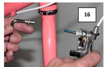
2 - On the brake pivot bolt there are two serrated washers. Remove both the serrated washers and insert the headlight bracket onto the brake pivot bolt, then replace one of the serrated washers. Now insert the brake bolt through the fender tab and insert the second serrated washer.
