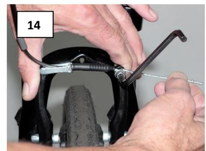
Be sure that the brake arms are evenly spaced from the wheel and there is some clearance between the brake pads and the rim surface. If the arms are not evenly spaced from the wheel, you can balance the spacing by gripping the brake assembly and rotating until it is centered with the wheel
