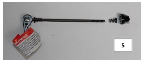
the conical spring (small side towards the axle) and screw on the adjusting nut with just a few turns. (**Figure 6**)
