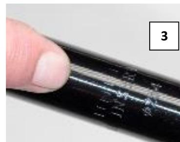
**WARNING!** *Using the bike with the minimum insertion line on the lower portion of the seat post showing above the frame could result in a failure of the seat post and/or the frame causing a loss of control with potential injury to rider. Such failures are not covered by warranty as it is improper use of the product.*
