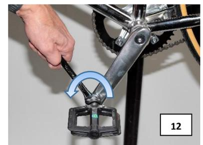
**NOTE:** *Be sure to tighten both pedals with an adjustable wrench or 15mm open end wrench to the recommended torque specification otherwise they will unscrew while riding causing an unsafe condition for the rider and damaging the threads in the crank.*
