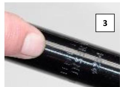
**WARNING!** *Using the bike with the minimum insertion line on the lower portion of the seat post showing above the frame could result in a failure of the seat post and/or the frame causing a loss of control with potential injury to rider. Such failures are not covered by warranty as it is improper use of the product.*
