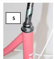
4. Adjust the height of the stem to your desired level and tighten the stem bolt using a 6mm wrench. You can make final adjustments to the height of the stem after the bike is assembled. **NOTE:** *Be sure that the minimum insertion mark on the shaft of the stem is inside the frame, it must not be visible outside of the frame (Figure 6).*
