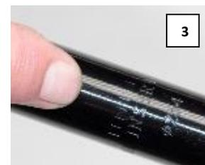
**WARNING!** *Using the bike with the minimum insertion line on the lower portion of the seat post showing above the frame could result in a failure of the seat post and/or the frame causing a loss of control with potential injury to rider.* Such failures are not covered by warranty as it is improper use of the product.
