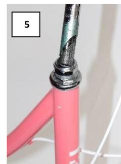
3 - Make sure that the fork is facing forward and the handlebars are lined up with the fork dropouts.
