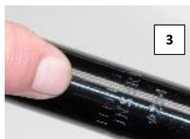
**WARNING!** *Using the bike with the minimum insertion line on the lower portion of the seat post showing above the frame could result in a failure of the seat post and/or the frame causing a loss of control with potential injury to rider.* Such failures are not covered by warranty as it is improper use of the product. (**Figure 3**)
