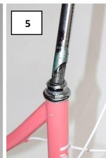
4. Adjust the height of the stem to your desired level and tighten the stem bolt using a 6mm wrench. You can make final adjustments to the height of the stem after the bike is assembled. NOTE: *Be sure that the minimum insertion mark on the shaft of the stem is inside the frame, it must not be visible outside of the frame. (Figure 6)*
