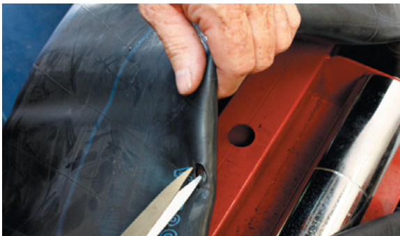
11. Move to the opposite side of the innertube and make a new hole to install the new valve.
