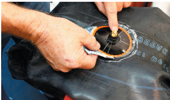
17. Line up the screw-on spud over the new hole and press firmly into place.
