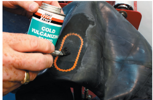
7. Cement buffed area including the buffed area of the first Repair Unit. Allow to dry.
