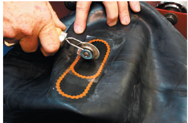
9. Stitch vigorously from the center out to remove any trapped air.
