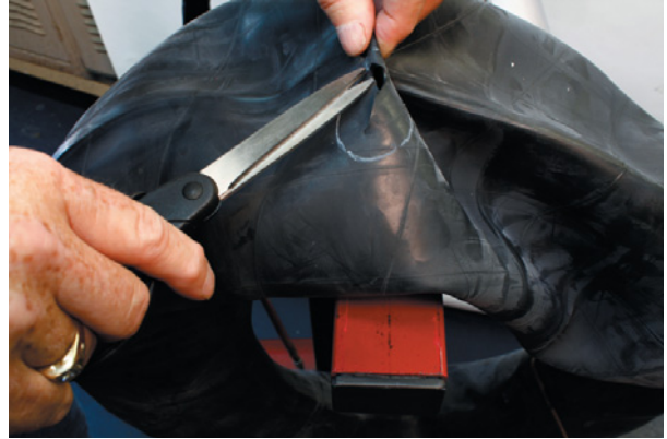
2. Round, or "button hole" the ends of the split
