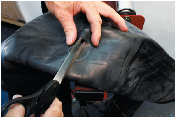
3. Trim a strip of rubber 1/16" of the length of the injury to prevent chaffing.
