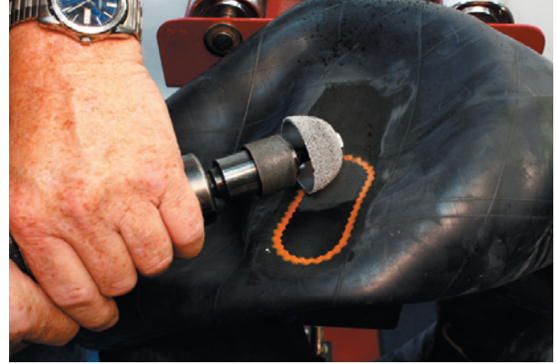
5. Buff remaining half of the injury as well as top half of applied Repair Unit.
