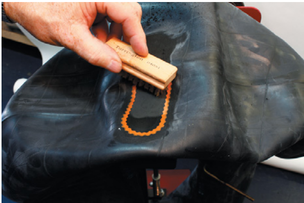
6. Clean the buffed area by using a brass brush.
