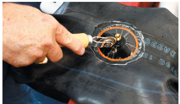
18. Stitch the base of valve thoroughly onto the inner tube starting in the center moving outward.
