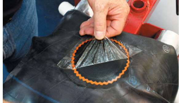
10. Remove the plastic from the top of the Repair Unit.
