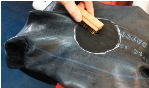
15. Clean the buffed area by using a brass brush.
