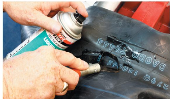
12. Use Pre-Buff Cleaner to clean the repair area. Spray and scrape the contamination from area.
