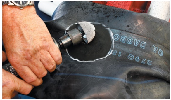
14. Using a low speed buffer, buff the desired area.
