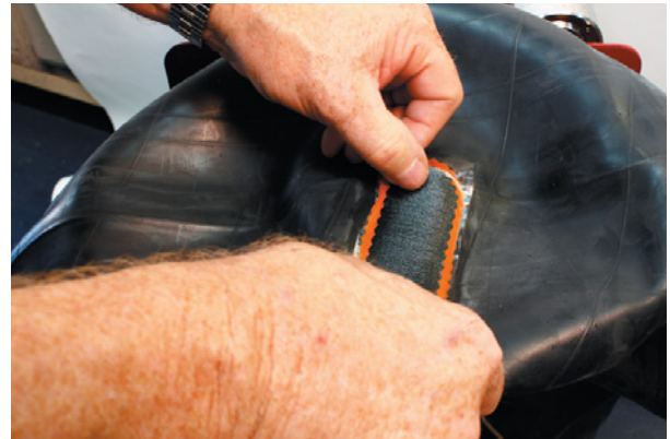
10. Remove the protective foil from the back of the Repair Unit and apply over the injury / cemented area. Avoid touching the Repair Unit.
