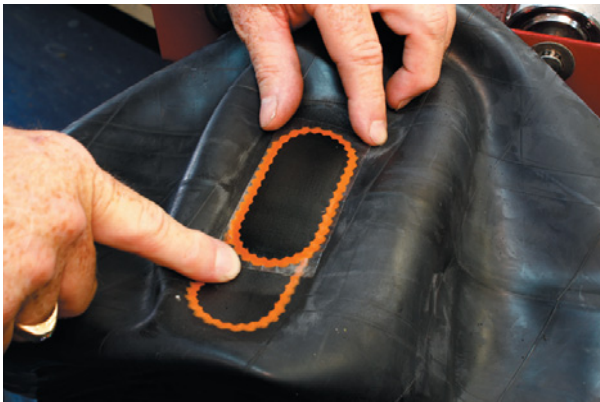
8. Remove the protective foil from the back of the Repair Unit and apply over the injury / cemented area. Avoid touching the Repair Unit.
