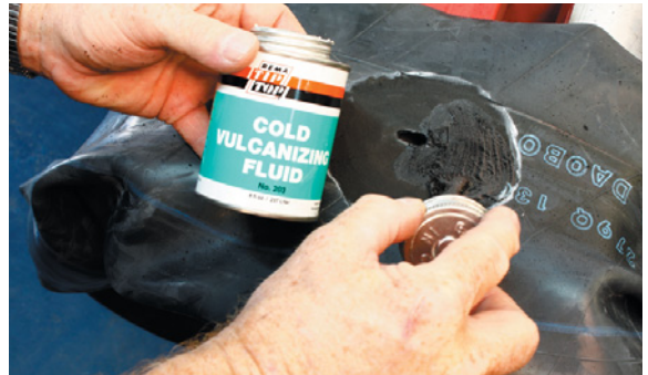
16. Apply a thin application of the proper cement and allow to dry.
