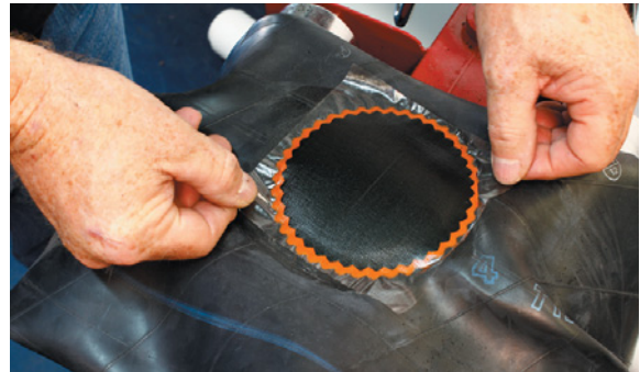
8. Remove the protective foil from the back of the Repair Unit and apply over the injury / cemented area. Avoid touching Repair Unit.
