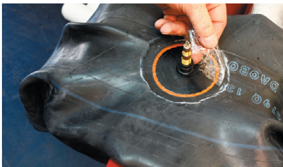
19. Screw on the appropriate spud and the repair is complete
