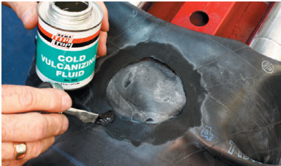
7. Apply a thin application of the proper cement and allow to dry.
