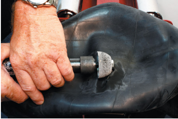
7. Using a low speed buffer (<5000rpm), buff the desired area.
