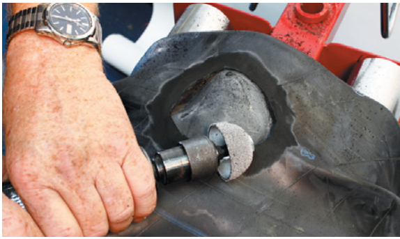
5. Using a low speed buffer, buff the desired area where the old valve was removed.
