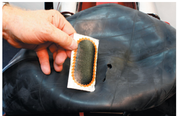
6. Select proper Tube Repair Unit. The Repair Unit should be approximately 1/2" larger than the prepared injury.
