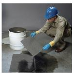
**Step 3:** When the pad or roll is fully saturated, simply pick it up and dispose of it. You'll know when it's fully saturated when you see liquids puddling around or passing underneath the sorbent. Don't forget to replace it with a fresh SpillTech sorbents.
