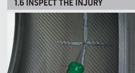
determine the extent of the damage and determine the inclination angle of the injury channel. easier insertion of the awl to inspect the injury.
