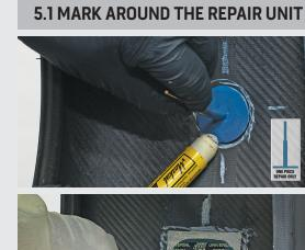
Center the repair unit over the injury and outline an area larger than the unit, so buffing will not remove the crayon
