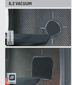
Use a vacuum to remove all debris from the inside of the tire. Do not touch the buffed area with the tip of the vacuum cleaner to avoid contamination. Always remove buffing dust with the use of a brass brush and vacuum. Never use compressed air. Do not use a Pre-Buff Cleaner on the buffed texture after you have buffed to avoid leaving residues which reduce adhesion.
