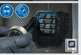
Check the repair area for defects. The finished repair should show no peeling or lifting at the edges, and should neatly Apply a generous application of 76F Innerliner Repair Sealant to the entire over-buffed area and the edge of the repair unit. If a MINICOMBI has been used, apply the Repair
