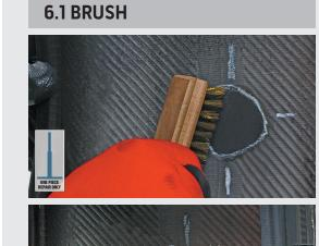
Clean the buffed area with a 6014 Brass Brush by brushing the area several times in one direction. Avoid brushing the non-buffed areas where there are contaminants that could be pulled onto the freshly buffed area. Use a brush that is designated only for tire repair and not used for anything else. This will help avoid contaminants in the buffed area.
