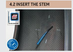
TWO PIECE REPAIR ONLY Remove the REMASTEM from the plastic packaging and place it in the pull wires (avoid touching the blue bonding layer when handling the REMASTEM). Fully coat the REMASTEM with cement and insert it into the eyelet of the pull wire. Insert the pull wire through the injury channel and auickly pull the pull wire through the tire. Pull until there
