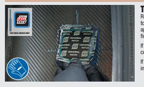
TWO PIECE REPAIR ONLY Remove the poly or foil from the back of the repair unit. Without touching the bonding layer, center the repair unit over the injury and apply carefully pushing down on the repair unit with your thumb or If using a directional repair unit, make sure to align the arrows in the
