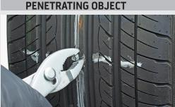
noting the direction of penetration. 1.5 MARK THE INJURY ON THE INSIDE
