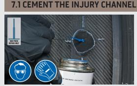
**ONE PIECE REPAIR ONLY** Apply BL-8F Special Blue Cement to the injury channel using a #626 pull-wire or a #190 awl. Special Blue Cement provides the necessary lubrication for the insertion of the repair unit, and bonds
