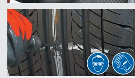
Determine the correct size Carbide Cutter from the NAIL HOLE REPAIR CHART above. Use a low speed tool (not to exceed 1200 rpm) to drill the injury from the inside out two or three times first and then from the outside in once or twice. Use full strokes with the carbide cutter, completely
