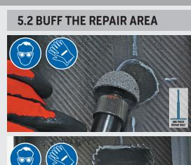
Lightly buff the repair area using a low speed (< 5,000 RPM) air or electric buffing tool with a clean buffing rasp, 36 to 60
