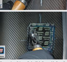
After the repair unit is applied, stitch thoroughly from the center outwards. Always start stitching from the center outward to remove any trapped air that may be under the repair unit. Continue several times in different directions over the whole surface of the repair unit to make sure that it is completely stitched to the innerliner and that it adheres securely to the buffed surface area.
