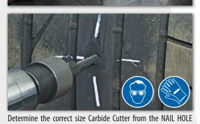
REPAIR CHART above. Use a low speed tool (not to exceed 1200 rpm) to drill the injury from the inside out two or three times first and then from the outside in once or twice. Use full strokes with the carbide cutter, completely removing the cutter from the tire
