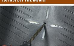
Inspect the injury with an awl, probing the injury to determine the extent of the damage and determine the inclination angle of the injury channel.
