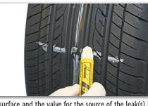
Check tire surface and the valve for the source of the leak(s) by using a leak detector. Mark the injury with a tire crayon.
