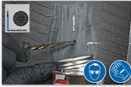
TWO PIECE REPAIR ONLY Apply PREMA PFC-8 Ultra Fast Dry Vulcanizing Cement to the injury channel using a PREMA Spiral Cementing Tool (PSCS).
