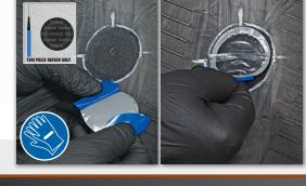
Remove the protective poly film from the Prema Repair Unit. NOTE: Take care not to touch the Gray Bonding Gum on the patch or stem of the repair unit.
