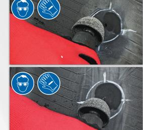
or electric buffing tool with a clean buffing rasp, 18 to 36 grit and remove all vent lines until you get a completely smooth surface. Continue lightly buffing the repair area to a smooth velvety finish (RMA Buff Texture 1 or 2) by putting slight pressure on the buffing tool and keeping it in constant movement.
