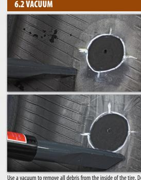
Use a vacuum to remove all debris from the inside of the tire. Do not touch the buffed area with the tip of the vacuum cleaner to avoid contamination. Always remove buffing dust with the use of a brass brush and vacuum. Never use compressed air. Do not use a Buffing Solution on the buffed texture after you have buffed to avoid leaving residues which reduce adhesion.
