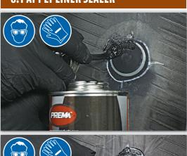
no peeling or lifting at the edges, and should neatly cover the repair area. Apply a generous application of PREMA PLOS-16 Innerliner Overbuff Sealant to the entire over-buffed area and the edge of the repair unit. If a Combi Repair Unit has been used, apply the
