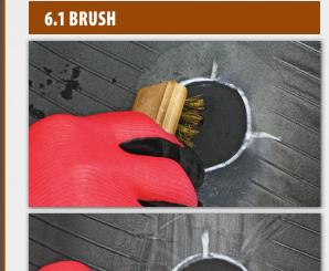
Clean the buffed area with a Brass Brush by brushing the area several times in one direction. Avoid brushing the non-buffed areas where there are contaminants that could be pulled onto the freshly buffed area. Use a brush that is designated only for tire repair and not used for anything else. This will help avoid
