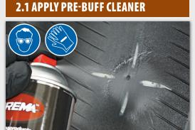
Apply PREMA PPC-16 Pre-Buff Cleaner around the injury area. Using an innerliner scraper, scrape the area to be buffed removing the contaminates such as dirt, tire lubes, and mold release lubricants. The area cleaned should be slightly larger than the selected repair
