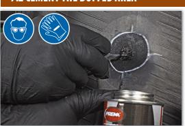
Apply a thin, even coat of PREMA PFC-8 Ultra Fast Dry Vulcanizing Cement to the buffed area of the tire innerliner using a clean brush. Use a swirling motion to apply the cement, as this will aid in the drying process as well as assure a thin, even coat. Completely cover the buffed
