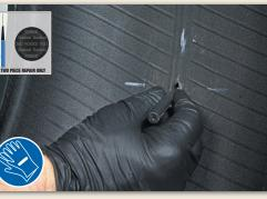
TWO PIECE REPAIR ONLY Fully coat the KEX Stem Unit with cement and guide the pilot wire of the KEX Stem Unit through the injury channel. Pull Stem Unit from the outside of the tire until there is approximately 1/4" (6 mm) of the stem remaining on the inside of the tire.
