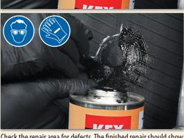
Check the repair area for defects. The finished repair should show no peeling or lifting at the edges, and should neatly cover the repair area. Apply a generous application of KX-508F Liner Sealer to the entire over-buffed area and the edge of the repair unit. If a Combi-Unit
