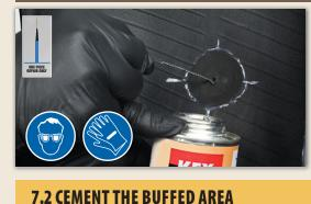
**ONE PIECE REPAIR ONLY** Apply KX-511F Super Fast Drying Cement to the injury channel using a #626 pull-wire or a #190 awl. Super Fast Drying Cement provides the necessary lubrication for the insertion of the repair unit, and bonds it
