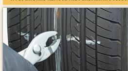
Locate and remove the penetrating object from the tire, noting the direction of penetration.
