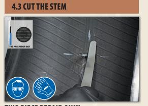
TWO PIECE REPAIR ONLY Cut the stem off leaving approximately 1/8" (3 mm) remaining on the inside of the tire. The remainder of the stem will be removed during the buffing process to provide a smooth surface.
