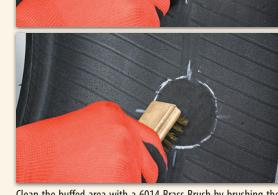
Clean the buffed area with a 6014 Brass Brush by brushing the area several times in one direction. Avoid brushing the nonbuffed areas where there are contaminants that could be pulled onto the freshly buffed area. Use a brush that is designated only for tire repair and not used for anything else. This will help avoid contaminants in the buffed area.
