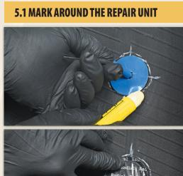
than the unit, so buffing will not remove the crayon marks. If the repair unit has bead arrows, make sure the arrows are
