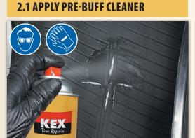
Apply KX-491F Buffing Solution around the injury area. Using an innerliner scraper, scrape the area to be buffed removing the contaminates such as dirt, tire lubes, and mold release lubricants. The area cleaned should be slightly larger than the selected repair unit. Scrape the innerliner while the Buffing Solution is still wet. Repeat 2-3 times until the surface is clean.
