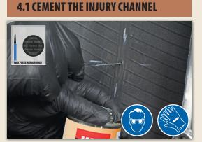
TWO PIECE REPAIR ONLY Apply KX-511F Super Fast Drying Cement to the injury channel using a #626 pull-wire or a #190 awl.
