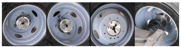
Mount chuck onto inside of wheel. Secure the Chuck by tightening with Ratchet Key. Verify you have full contact on the wheel surface of all 3 jaws. Lift wheel and tire and mount the Chuck onto balancer shaft. Push the tire all the way back. Place the clamping cup over balancer shaft, and secure with wing nut.
