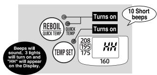
The Automatic Shut-Off function activates to shut down power to the heater in order to prevent damage from overheating. The Display will show "HH" and beeps will sound to alert you that the Automatic Shut-Off has been activated. The following conditions may cause activation:
